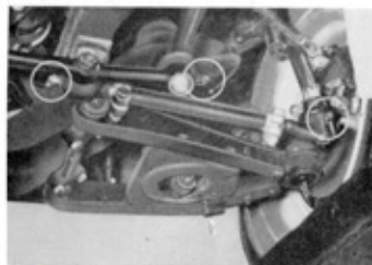
Tie Rod Center Link Chassis Grease Supply every 6,000km
